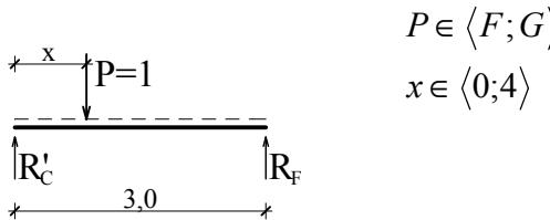
$$\begin{aligned}\sum M_F &= 0 \\ Px - 4R_G &= 0 \\ R_G &= \frac{x}{4}\end{aligned}$$
